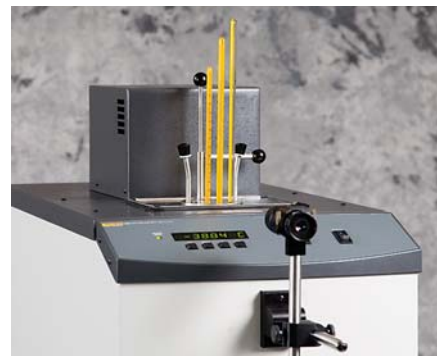
The 2019-DCB Liquid-in-Glass Thermometer Calibration Kit includes a carousel which holds up to 10 thermometers and an adapter tube which raises the bath fluid level to within 5–15 mm of the thermometers' readings. The 2069 Magnifier Scope mounts easily to the front of any Deep-Well Compact Bath to provide magnification of 8X or greater.
