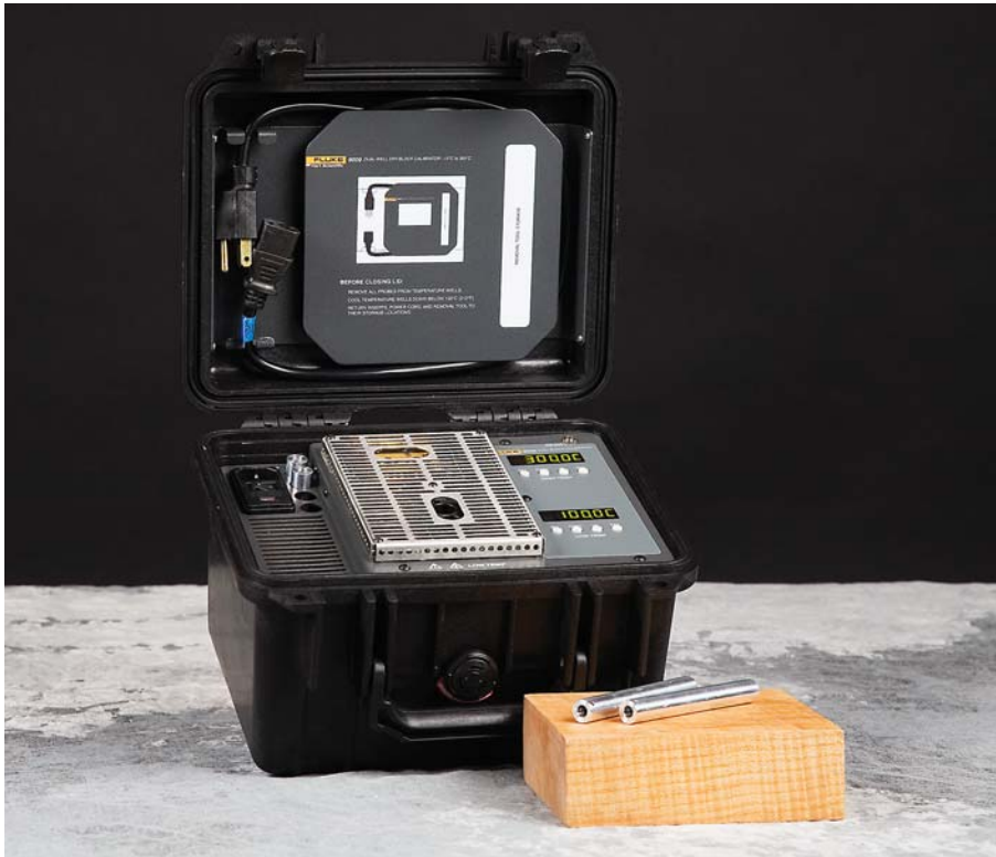
Each block contains two wells, which accept removable inserts. A 1/4" and a 3/16" insert are included for each block. Additional sizes (including custom sizes) are available.
